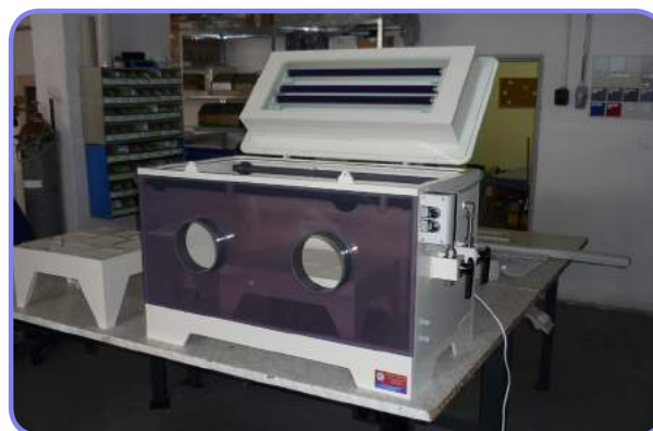
Figure 3. Test chamber developed at ICT Prague. Test materials held on tables are exposed to UVA from above. The illustration shows the chamber with the lid, holding the UVA lamps, open. Gloves attached to the two ports enable aseptic handling of contaminated test surfaces in the chamber.
